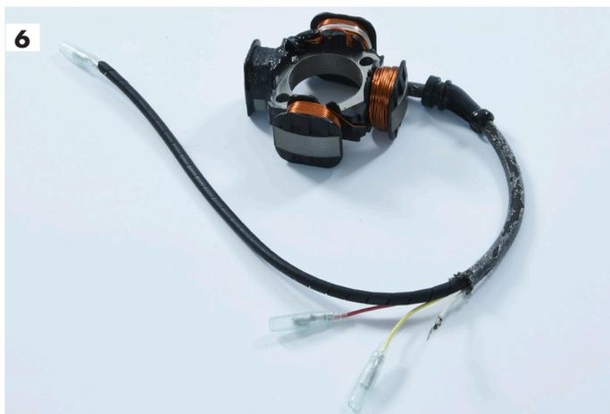
Fix the stator using 2 screws M5x25 with their washers ( photo 7).
