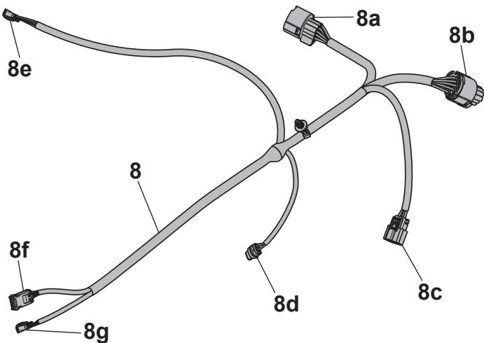
Starting from the right side of the vehicle, pass the part of the wiring harness **8** containing the connectors **8d / 8e / 8f / 8g** under the bracket of the device towards the left side of the vehicle, taking care to hook the clamp on the wiring harness into the appropriate hole in the bracket, as shown in the figure.
