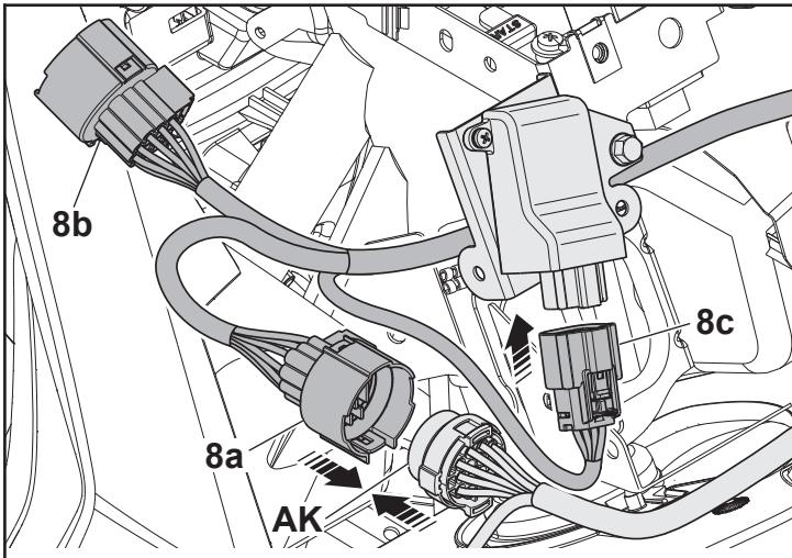
**G** Connect the connector **8a** of the wiring harness **8** to the connector **AK** of the vehicle wiring harness and the connector **8c** to the heating accessories device.
