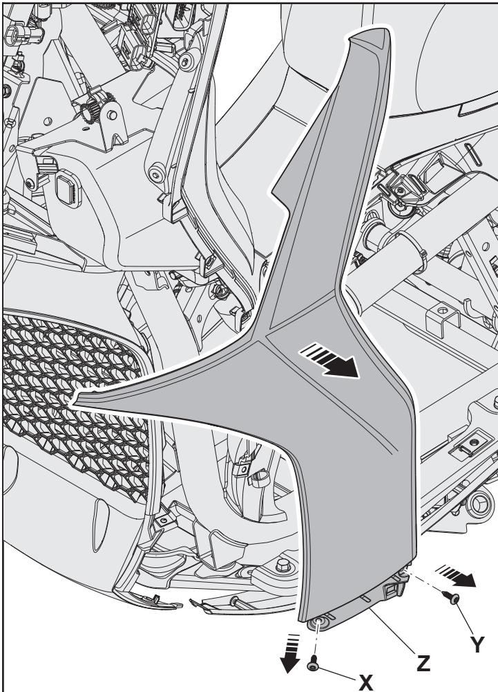
**G** Remove the screw **X**, the screw **Y** and the left side fairing **Z**.
