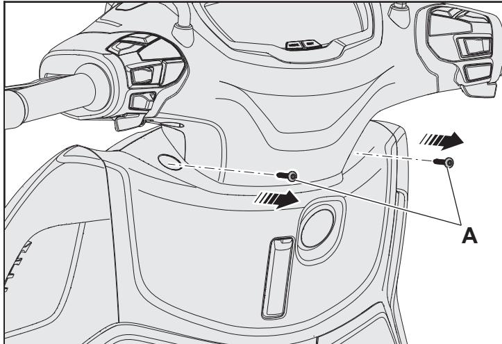
Remove the screws **A** from the upper part of the shield.
