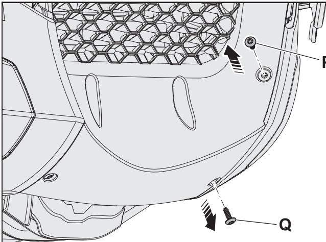
**G** Remove the screw **P** and screw **Q** from the lower left of the front wheel arch.
